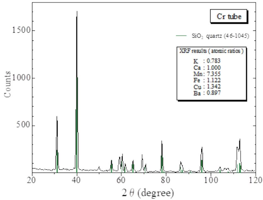
Fig.34 XRD spectrum taken from the cross section of the ornament
