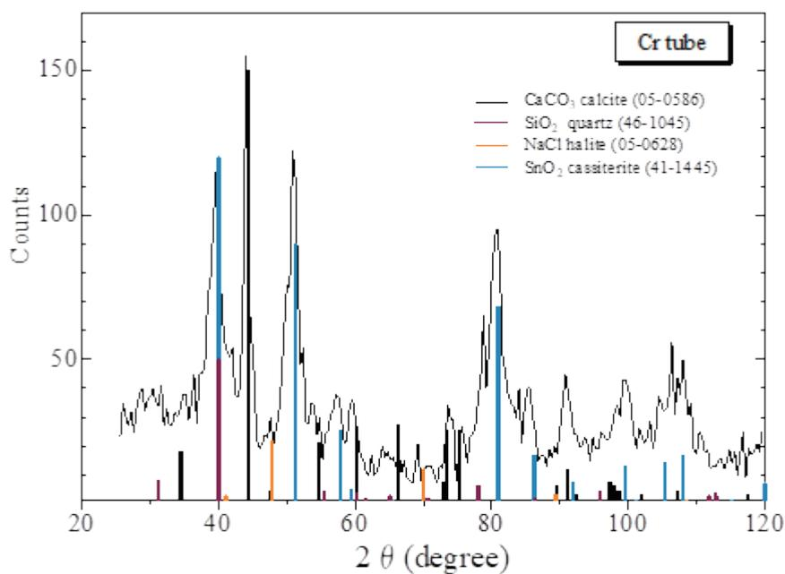
Fig.40 XRD spectrum taken from a gray face
