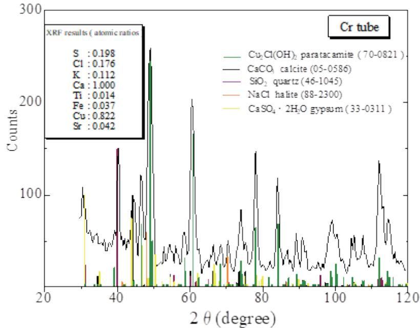
Fig.38 XRD spectrum taken from a green part
