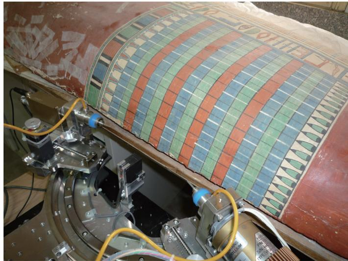
Fig.36 X-ray analysis for colored parts of the garment
