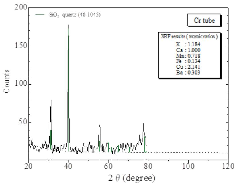
Fig.35 XRD spectrum taken from the surface of the ornament
