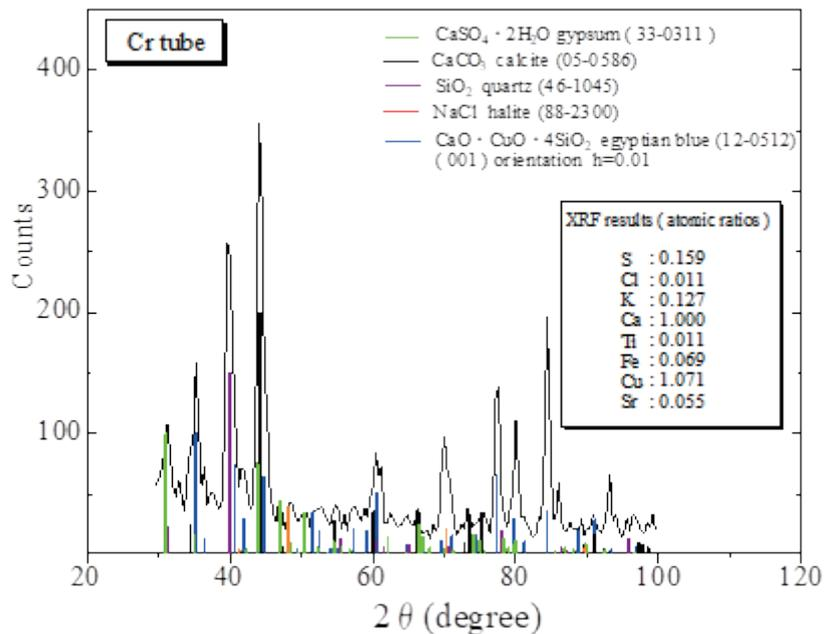
Fig.37 XRD spectrum taken from a blue part
