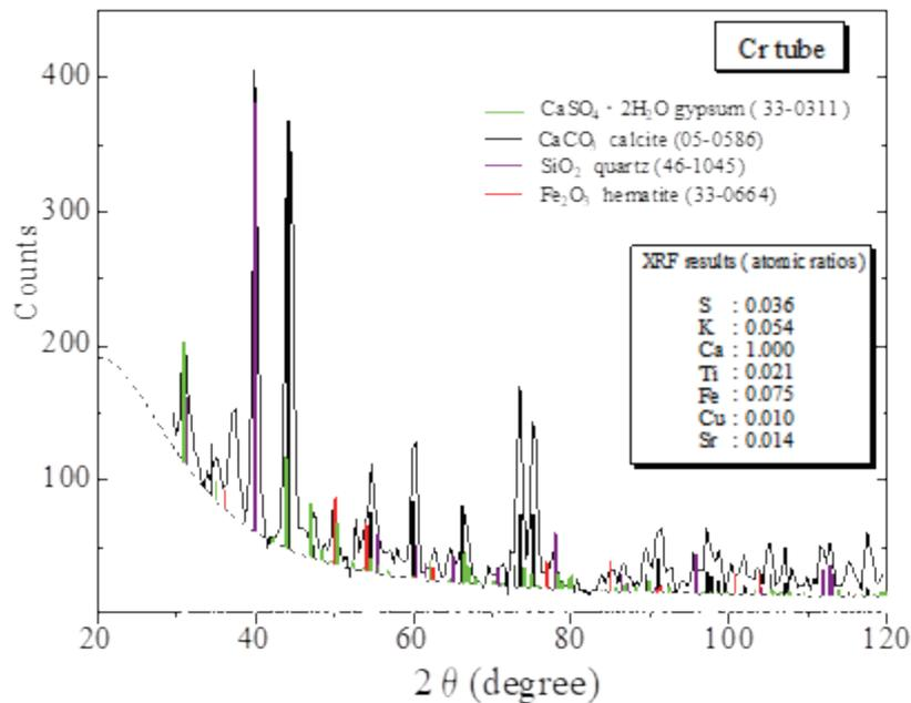
Fig.39 XRD spectrum taken from a red part
