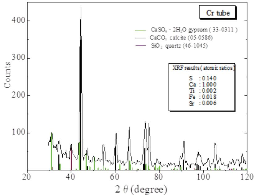
Fig.40 XRD spectrum taken from a white part
