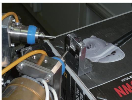
Fig.33 X-ray Analysis on a broken ornament
